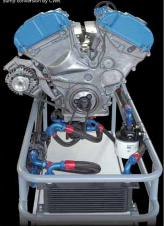
Ford Duratec V6 demo with ARE Dry Sump conversion by CWR.
